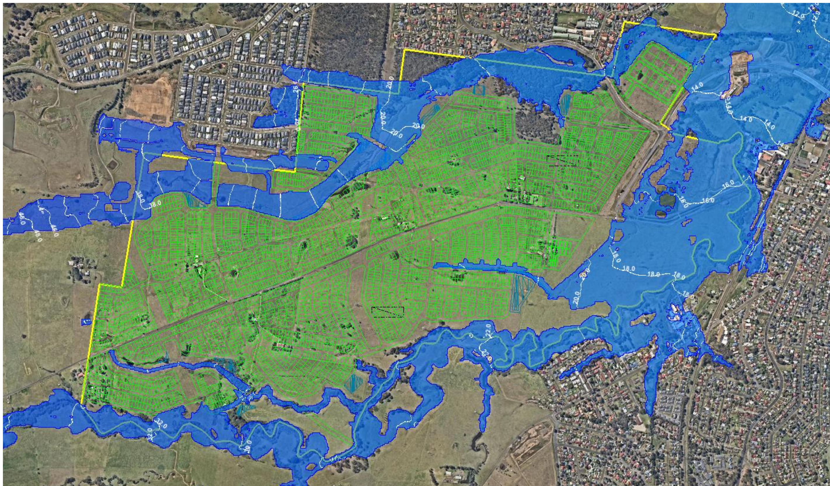
Figure C2.1: 1% AEP Flood Levels – Post-Development
